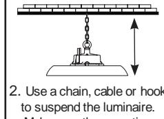
2. Use a chain, cable or hook to suspend the luminaire. Make sure the mounting hardware is securely attached to a stationary structure and strong enough to safely suspend the luminaire.
